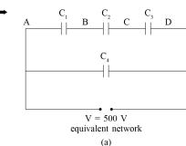
(a) For the given network, (fig.a) all 3 capacitors  $C_1$ ,  $C_2$  and  $C_3$  are in series connection, and their effective (/ equivalent) capacitance is C'.
